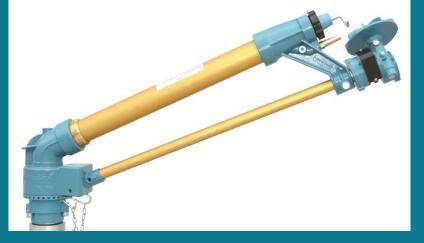
Run length: 300m Working Pressure: 40 - 90 psi Water Flow: 300 - 750 l/min Effective Spray Width: 50 - 90 m Sprinkler : DuCaR Jet 55
